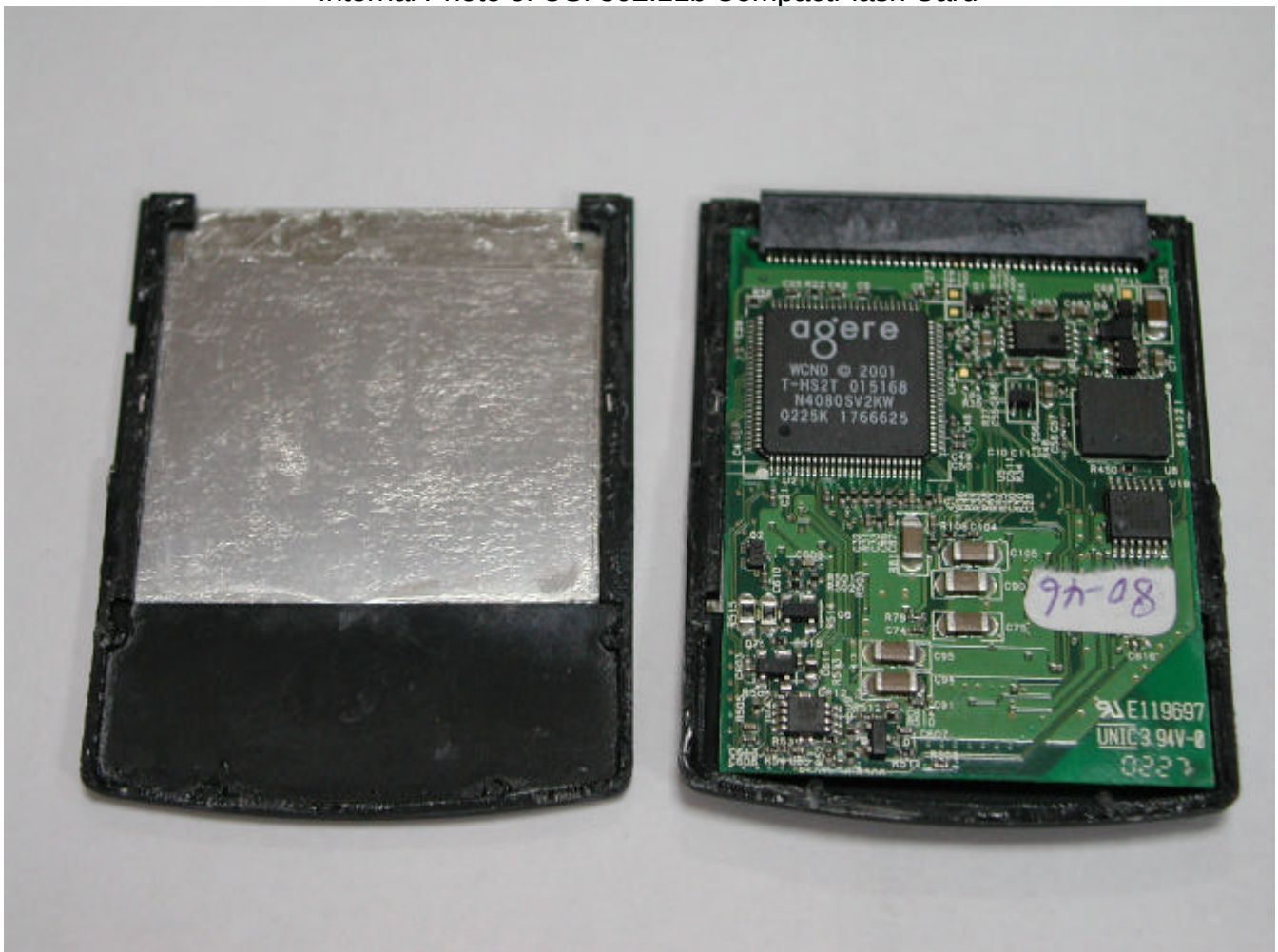
Internal Photo of USI 802.11b CompactFlash Card
