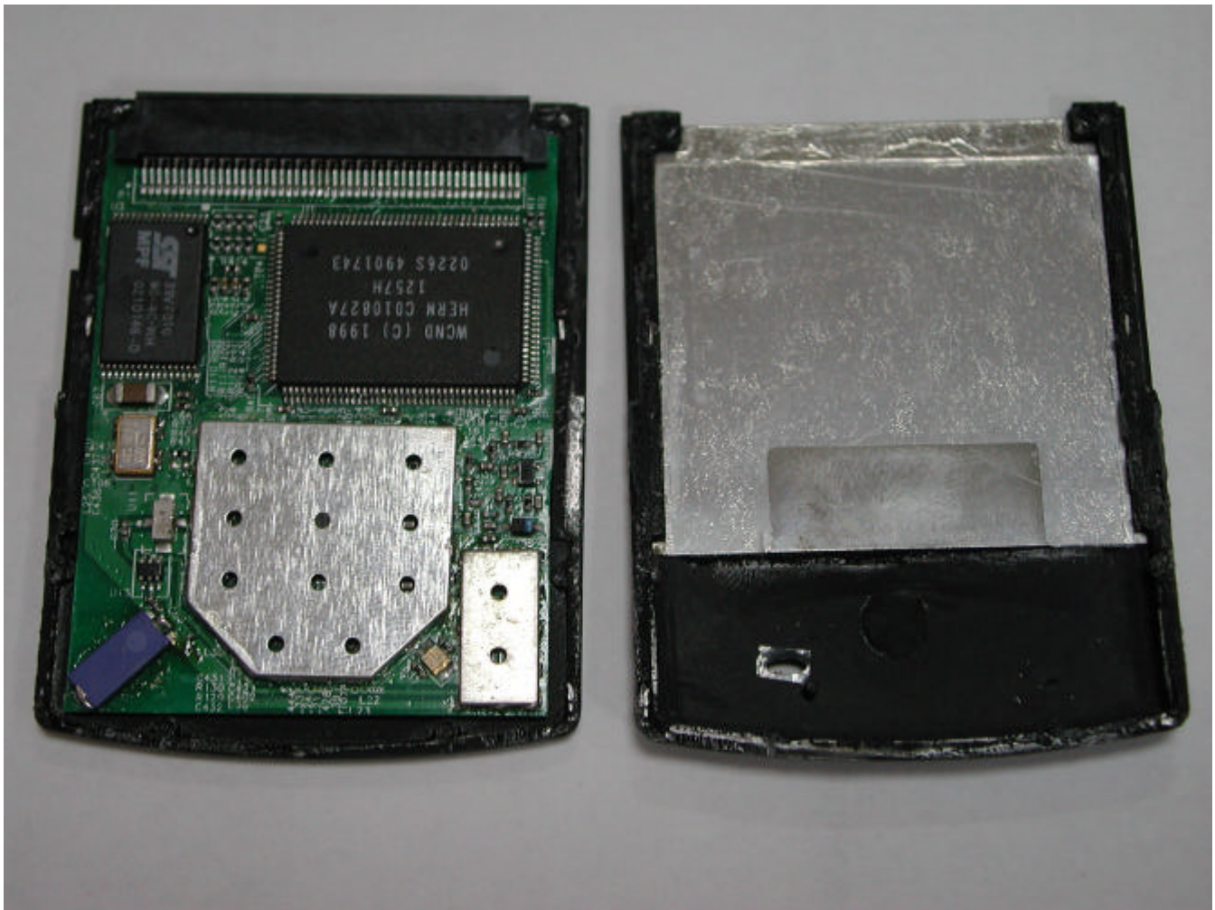
Internal Photo of USI 802.11b CompactFlash Card
