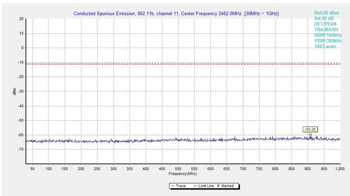
Fig.B.6.1.18 Transmitter Spurious Emission - Conducted (802.11b, Ch11, 30 MHz-1 GHz)
