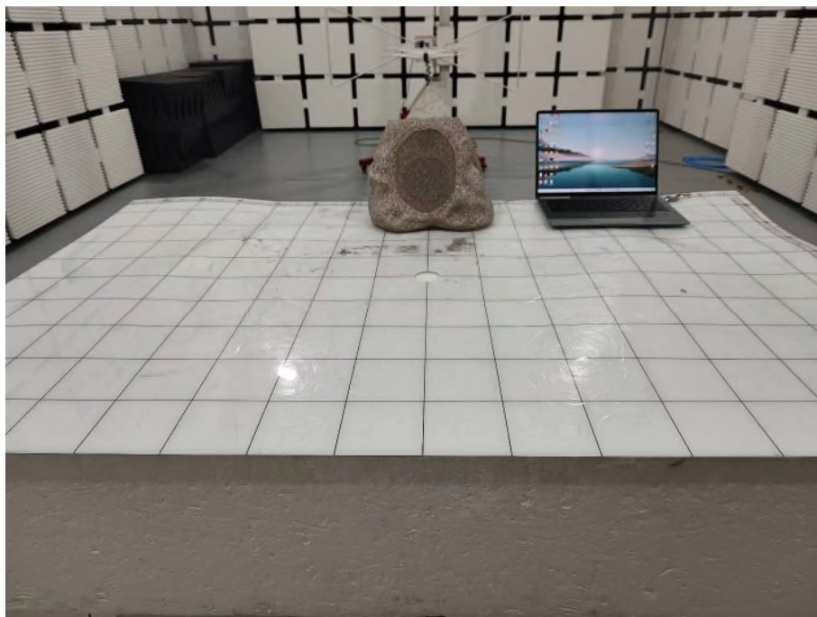
Photograph 1: Set-up for Radiated Spurious Emission, 30MHz - 1GHz
