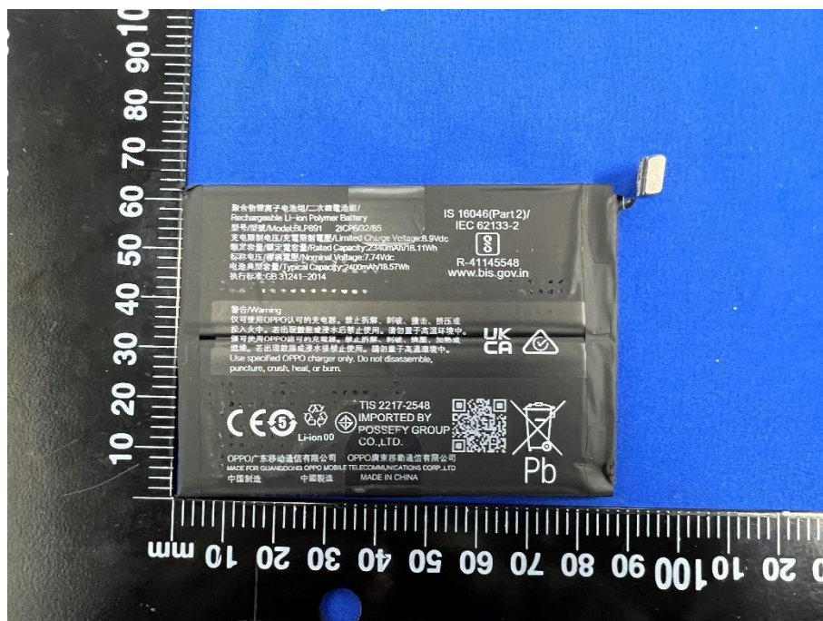
Battery Photo (FRONT)
