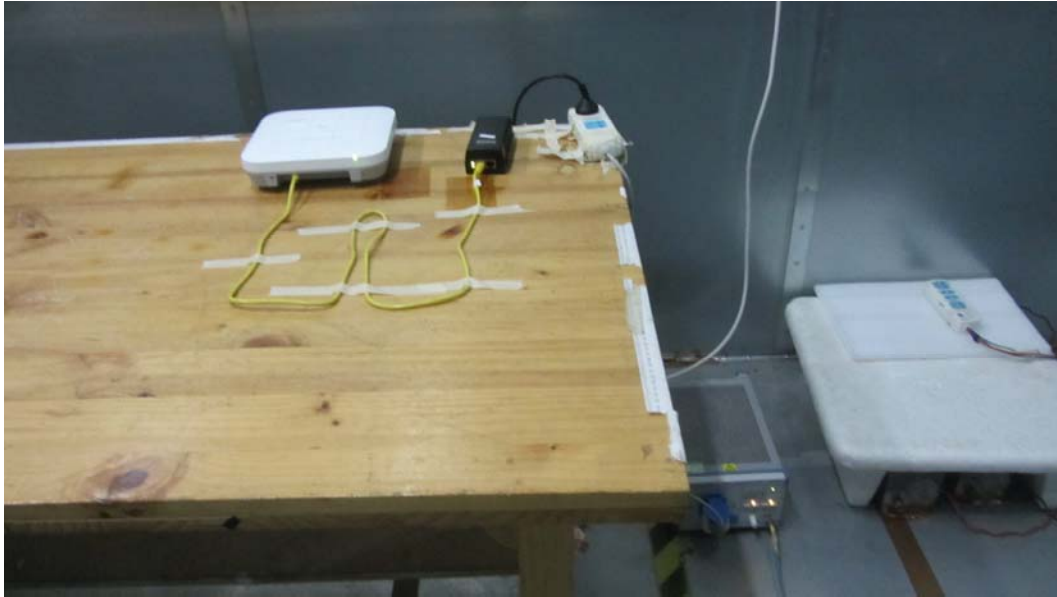
Picture 3 Conducted Emission Test Setup
