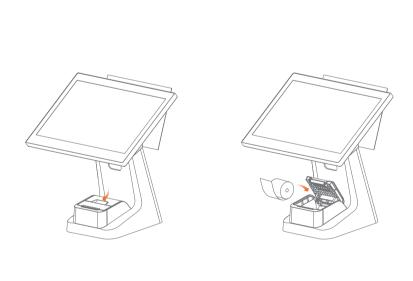
As shown in the figure, press the button at the bottom left corner to pop open the printer cover.
