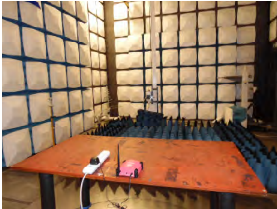
Photograph 2: Set-up for Radiation Measurement above 1GHz
