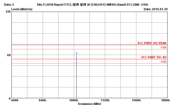
Remarks: 1. Emission Level= Antenna Factor + Cable Loss + Reading -Amp factor.
