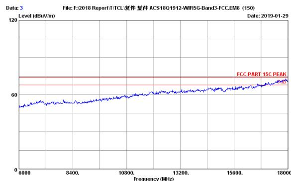
Remarks: 1. Emission Level= Antenna Factor + Cable Loss + Reading -Amp factor.
