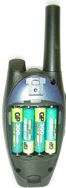
DUT with NiCd Batteries
