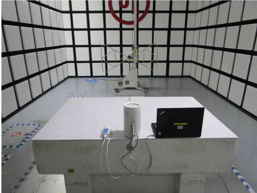
POWERLINE CONDUCTED EMISSIONS MEASUREMENT SETUP
