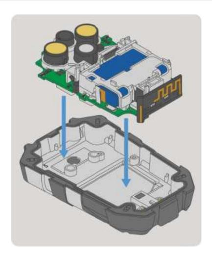
(7) Install the main board into the replacement back housing.
