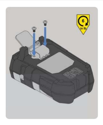
(5) Install the two screws with a Phillips head #1 screwdriver. Torque to 6 in-lbs (0.68 N-m).
