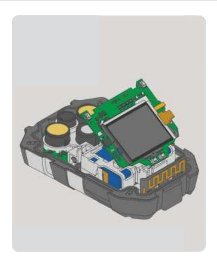
(3) Remove the display PCBA and display assembly by lifting it up.
