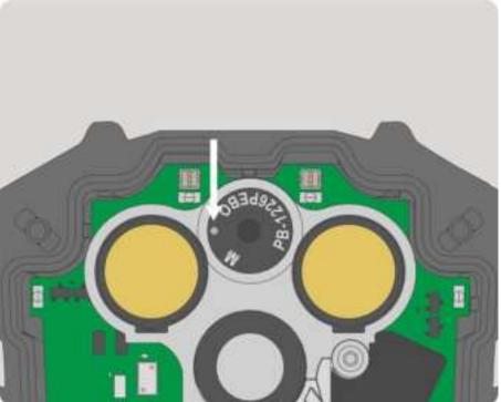
(4) Install the replacement horn by pushing it down into the clear bracket.
