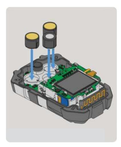
(4) Install the replacement sensor(s) by pushing it down into the clear bracket.
