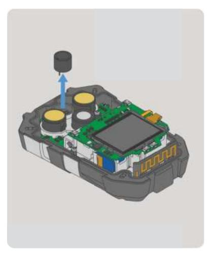
(3) Remove the horn by pulling it up and out of the clear bracket.
