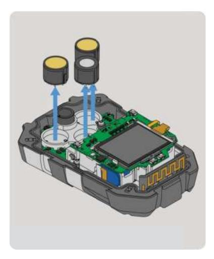
(3) Remove the sensor(s) you plan on replacing by pulling it up and clear of the bracket.
