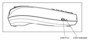
LED indicator: Power status indicator of device USB Port: USB communication interface
