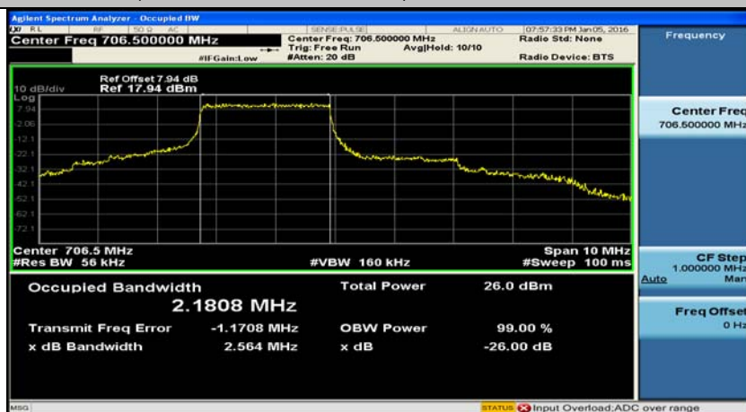
(Channel Bandwidth: 5 MHz)_LCH_QPSK_12RB#6
