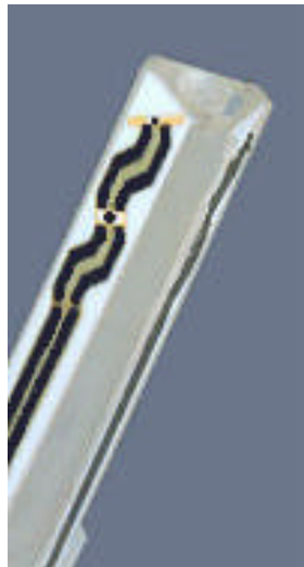
Fig. 5. ET3DV5 E-field Probe
