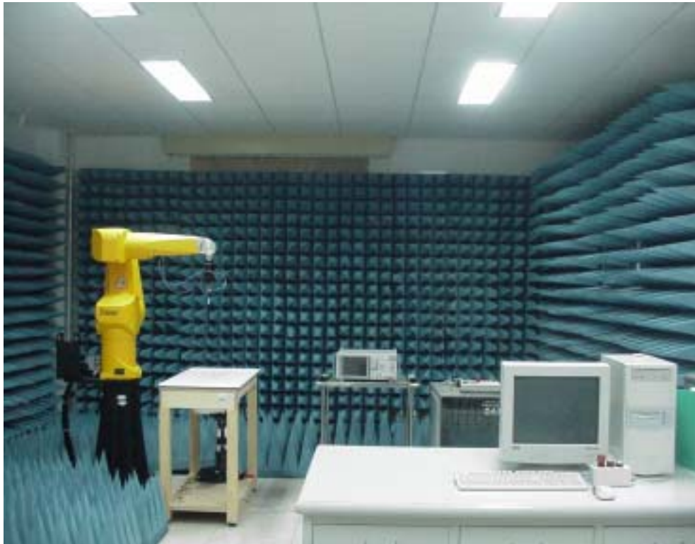
Picture 1 Specific Absorption Rate Test Layout
