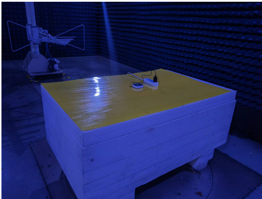
Photo of Radiated Emission Measurement (Below 1G)
