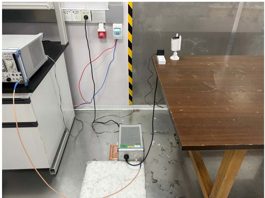
Conducted Emission Test Setup
