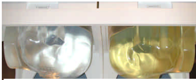
Figure 7.1 Left and Right SAM Phantom shells
