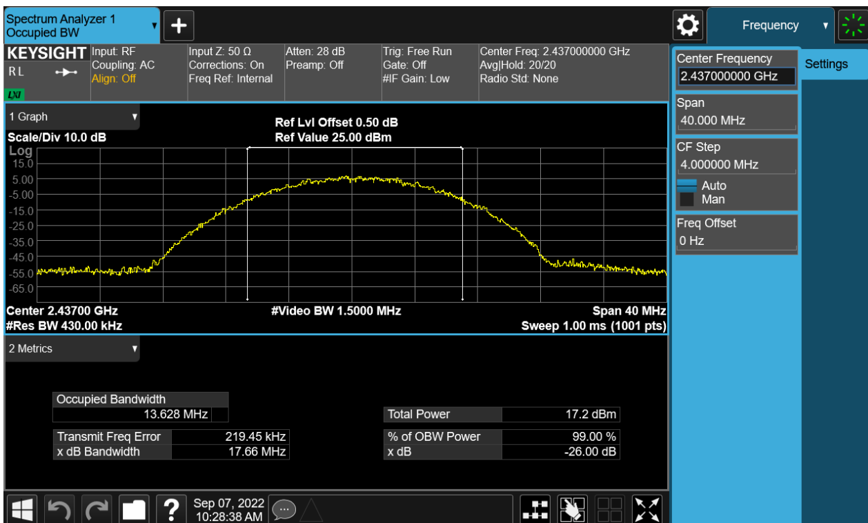
Figure 4: The plots of 99% Bandwidth, 802.11b, 2437MHz
