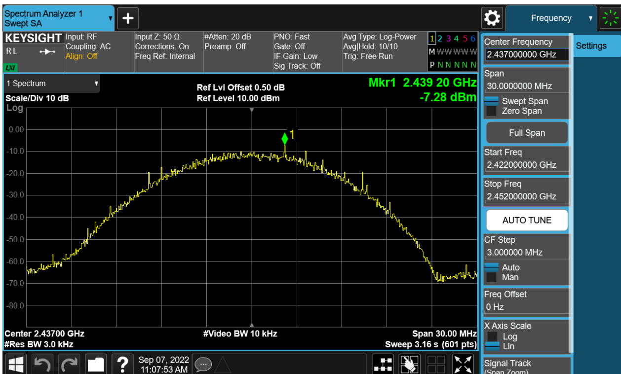
Figure 38: The plots of Power Spectral Density, 802.11b, 2437MHz, Chain 2
