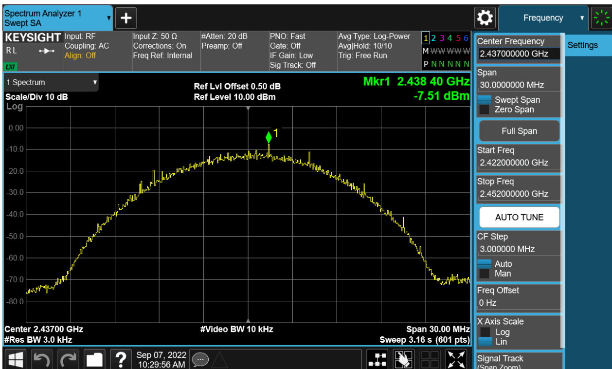
Figure 26: The plots of Power Spectral Density, 802.11b, 2437MHz, Chain 1
