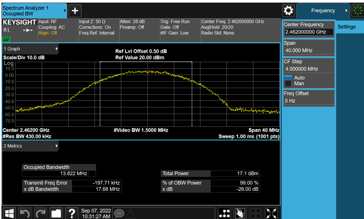
Figure 6: The plots of 99% Bandwidth, 802.11b, 2462MHz
