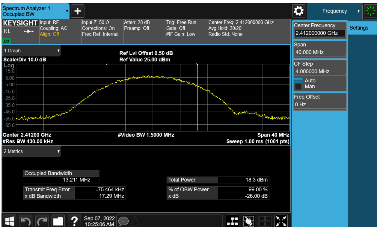
Figure 2: The plots of 99% Bandwidth, 802.11b, 2412MHz
