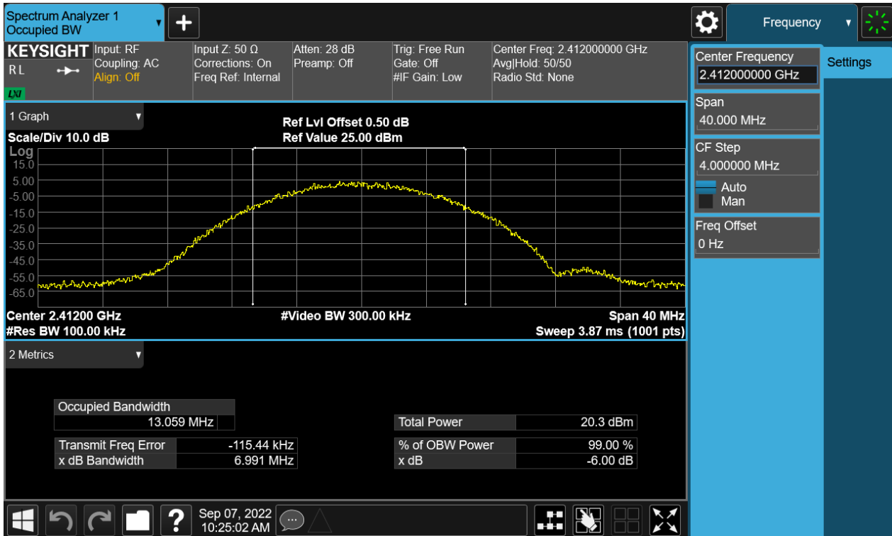
Figure 2: The plots of 99% Bandwidth, 802.11b, 2412MHz
