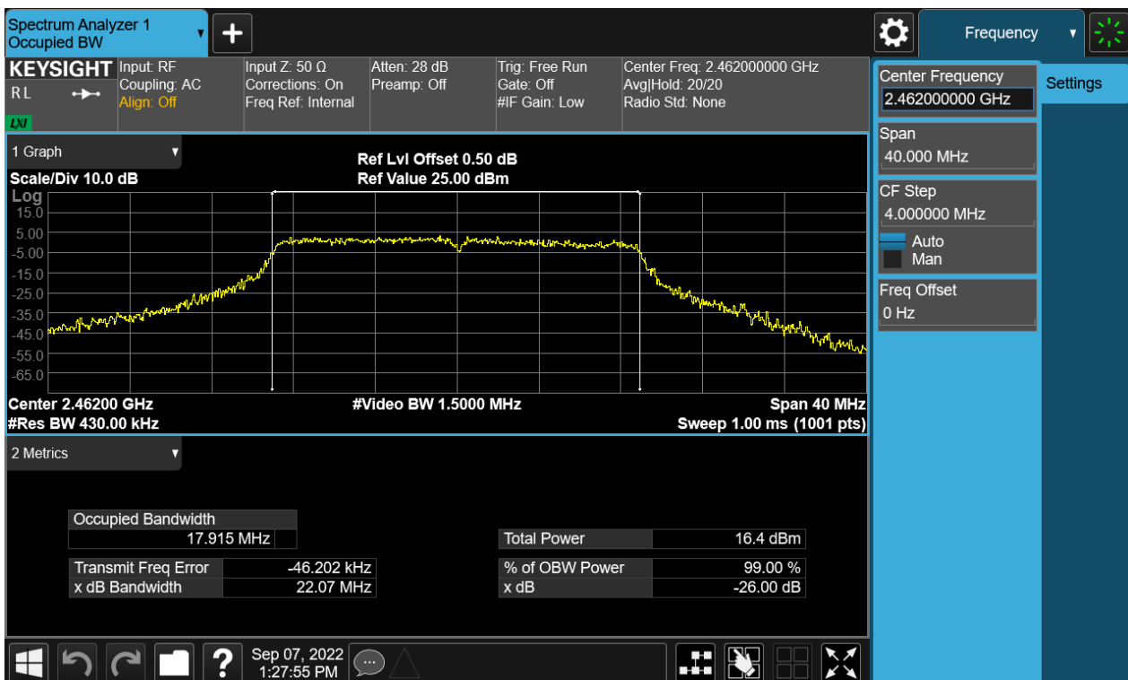
Figure 18: The plots of 99% Bandwidth, 802.11n(HT20), 2462MHz
