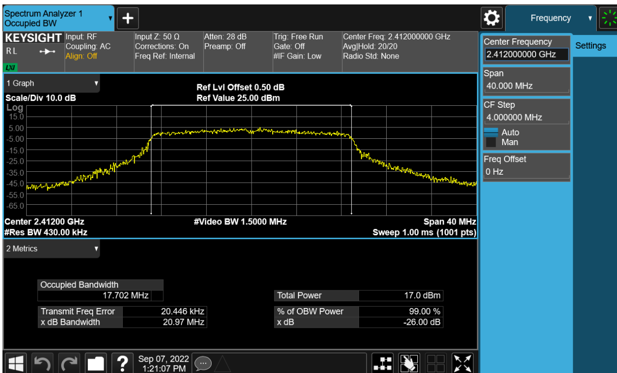
Figure 14: The plots of 99% Bandwidth, 802.11n(HT20), 2412MHz
