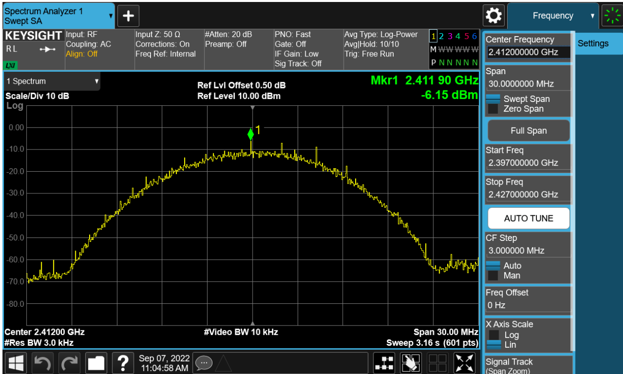
Figure 38: The plots of Power Spectral Density, 802.11b, 2437MHz, Chain 2
