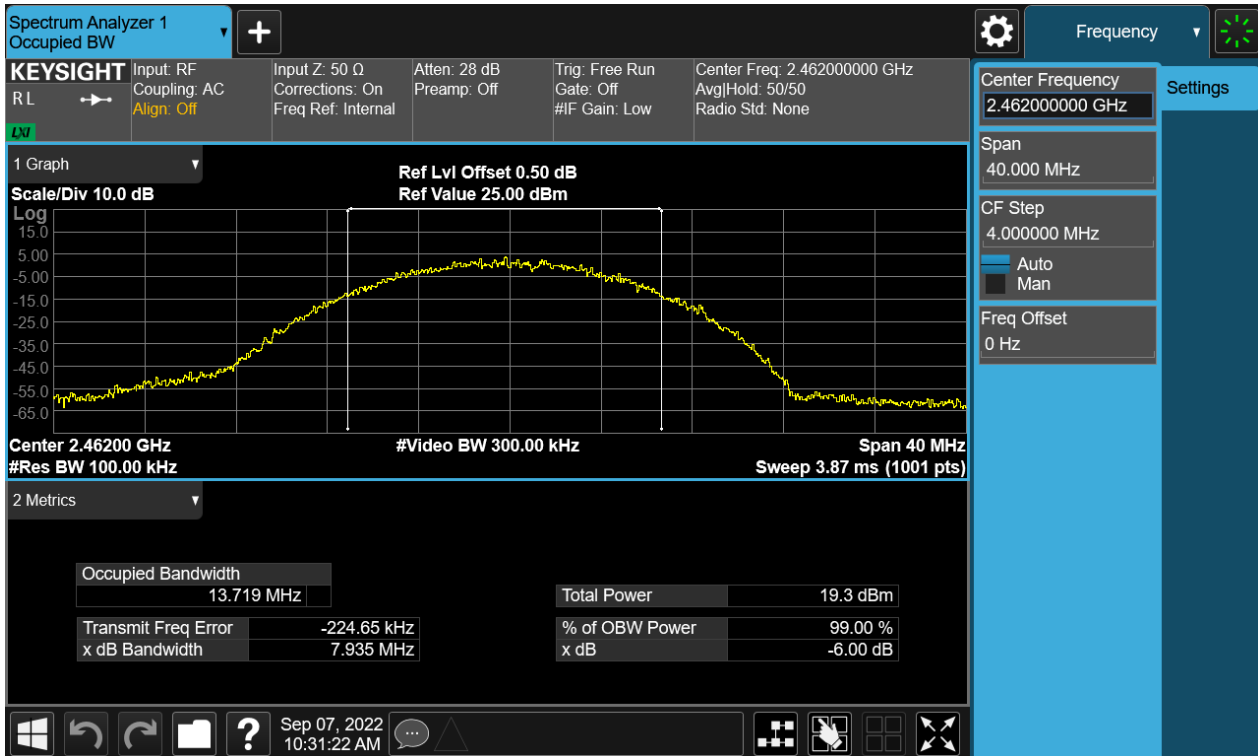
Figure 6: The plots of 99% Bandwidth, 802.11b, 2462MHz
