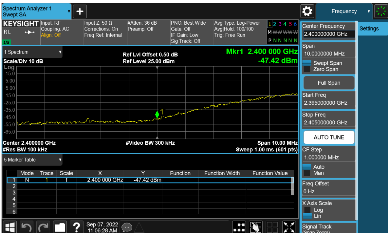
Figure 50: The plots of Conducted Spurious Emission & Authorized-band band-edge, 802.11b, 2412MHz Band Edge
