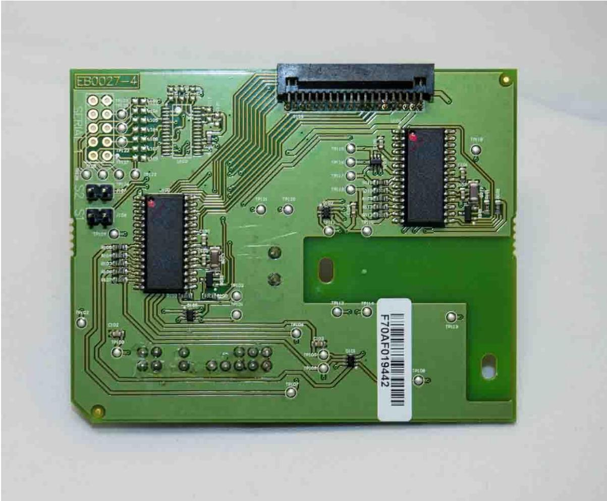
Figure 22 UPC SAM board bottom
