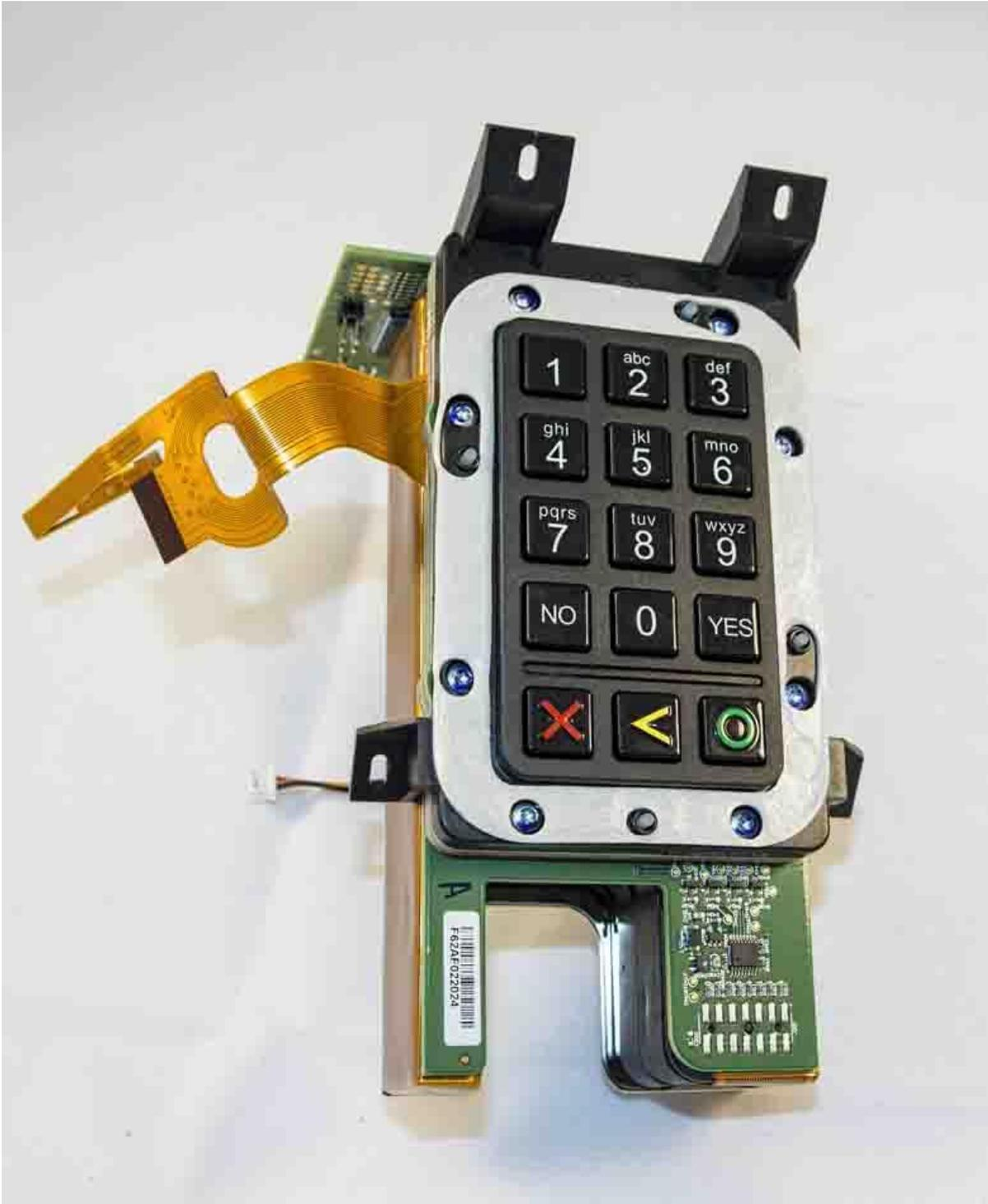
*Figure 17 Unified Pin-pad and Card reader*
