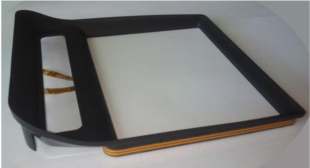
*Figure 1 Bezel removed showing Contactless Circuit Antenna (Bezel up- Normal position)*
