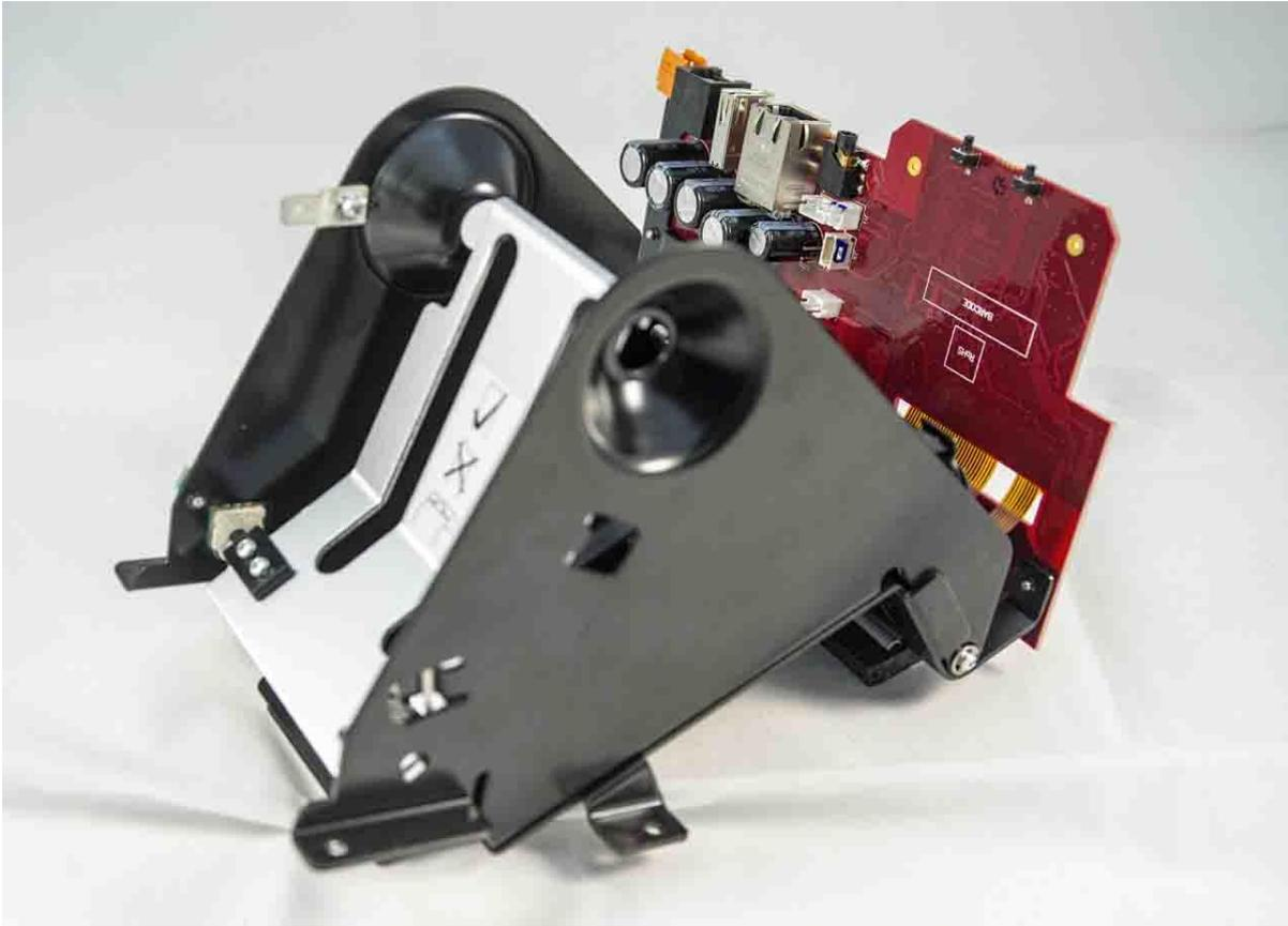
*Figure 6 Printer chute and power supply board*
