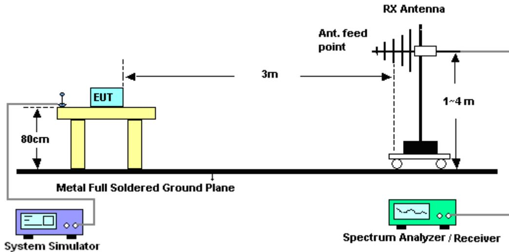
For radiated test above 1GHz
