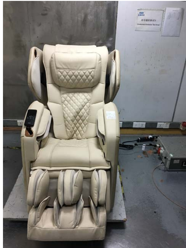
Photograph of set-up for conducted Emission
