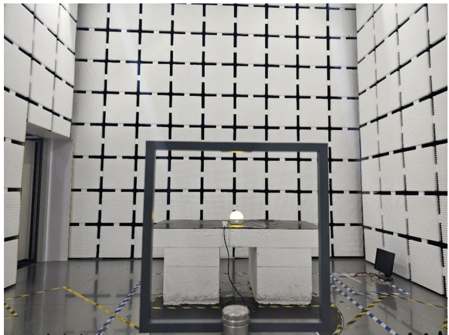
Radiation Emission Test Setup (Below 30MHz)
