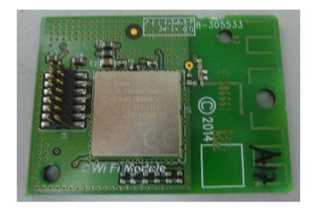
Photograph No.12 Control panel Wi-Fi module second side view
