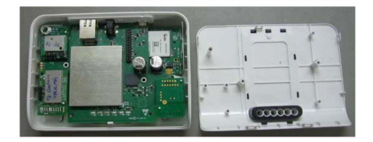
Photograph No.2 "PM-360 (433) ADT" control panel PCB front view
