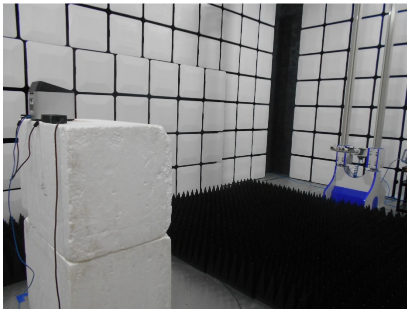
Photo 1.3-3 – RE Spurious Emissions 18-40 GHz
