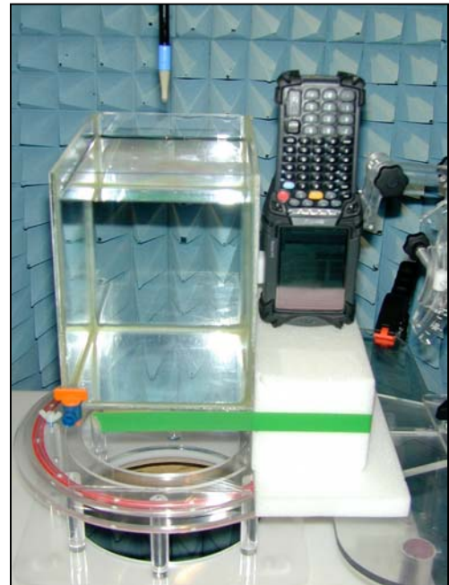
Figure 40. Positional photograph of the MC9062 Right-hand side at 1.0cm from Phantom side
