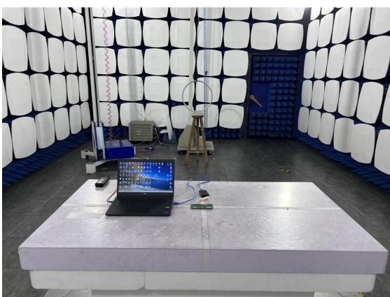
3. Radiated emission (9KHz-30MHz)
