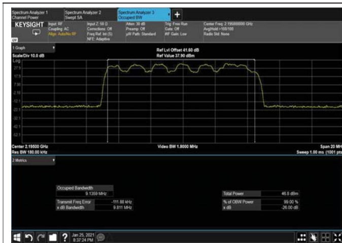
Figure 313: QPSK 10MHz B.W; 2195MHz, 15kHz OUTPUT
