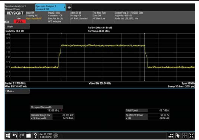
Figure 298: 256QAM 15MHz B.W; 2117.5MHz, 30kHz OUTPUT
