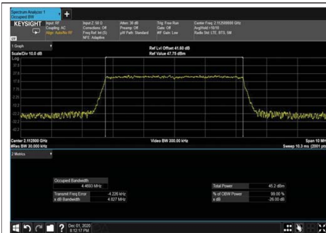
Figure 354: 16QAM 5MHz B.W; 2112.5MHz – 4G OUTPUT
