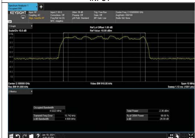
Figure 179: 16QAM 5MHz B.W; 2155.0MHz, 15kHz INPUT
