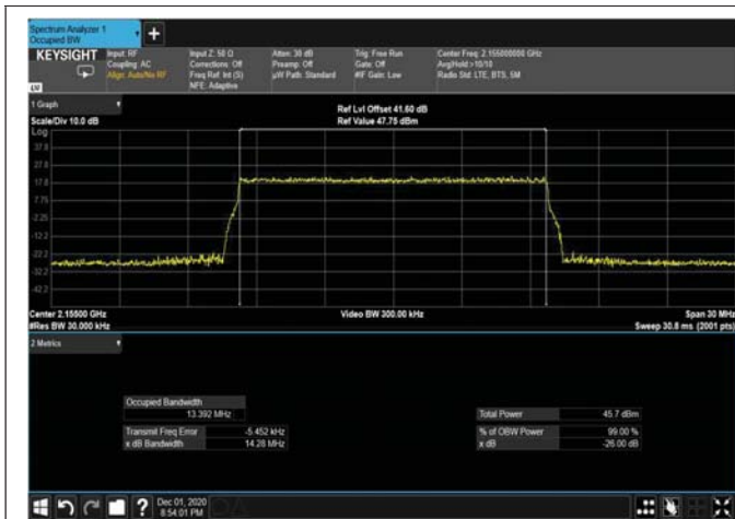
Figure 370: 64QAM 15MHz B.W; 2155MHz – 4G OUTPUT
