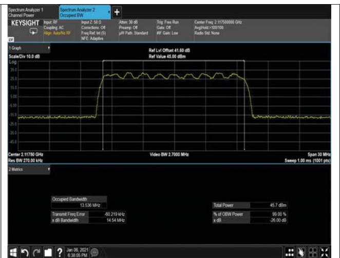
Figure 262: 16QAM 15MHz B.W; 2117.5MHz, 30kHz OUTPUT
