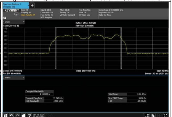
Figure 236: QPSK 5MHz B.W; 2197.5MHz, 30kHz INPUT
