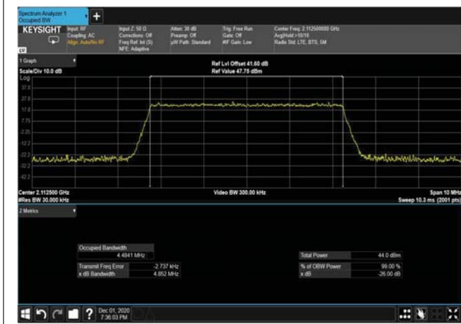
Figure 372: QPSK 5MHz B.W; 2112.5MHz – 4G OUTPUT
