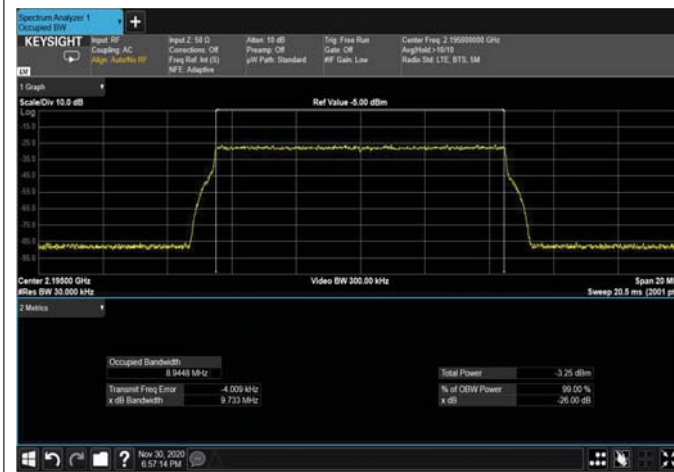
Figure 338: 64QAM 10MHz; 2195MHz – 4G INPUT
