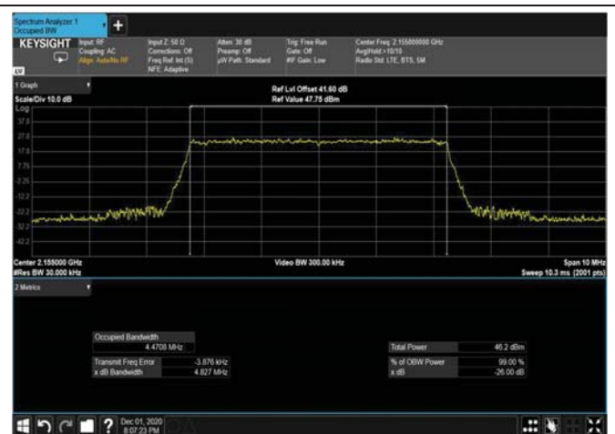
Figure 355: 16QAM 5MHz B.W; 2155MHz – 4G OUTPUT
