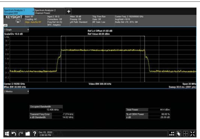
Figure 371: 64QAM 64MHz B.W; 2192.5MHz – 4G OUTPUT
