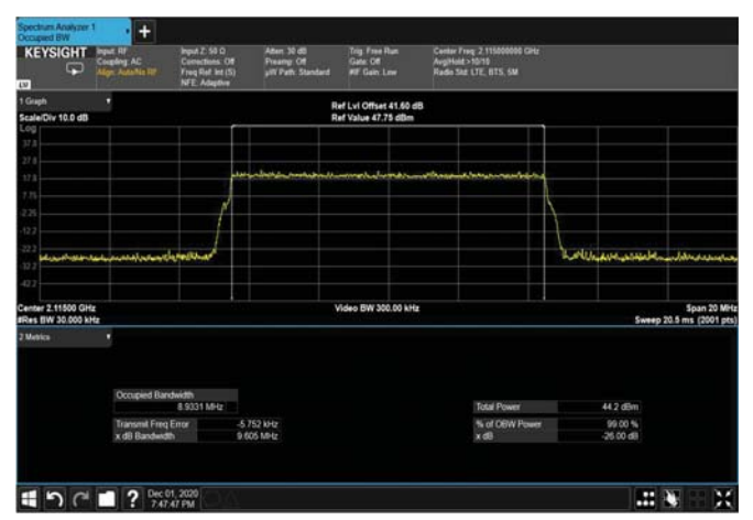
Figure 375: QPSK 10MHz B.W; 2115MHz – 4G OUTPUT
