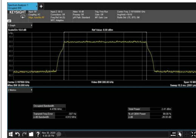
Figure 344: QPSK 5MHz B.W; 2197.5MHz – 4G INPUT
