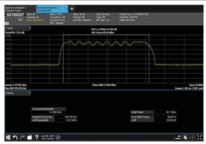
Figure 316: QPSK 15MHz B.W; 2117.5MHz, 30kHz OUTPUT
