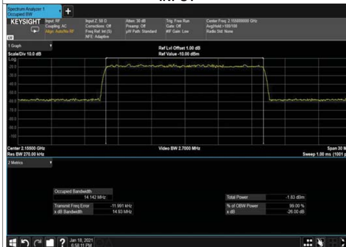
Figure 209: 64QAM 15MHz B.W; 2155.0MHz, 15kHz INPUT
