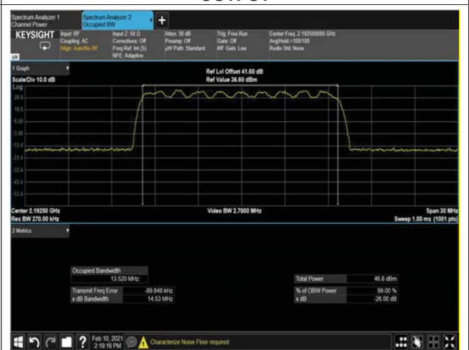
Figure 266: 16QAM 15MHz B.W; 2192.5 MHz, 30kHz OUTPUT
