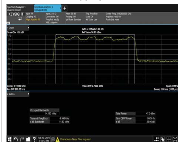
Figure 265: 16QAM 15MHz B.W; 2192.5 MHz, 15kHz OUTPUT
