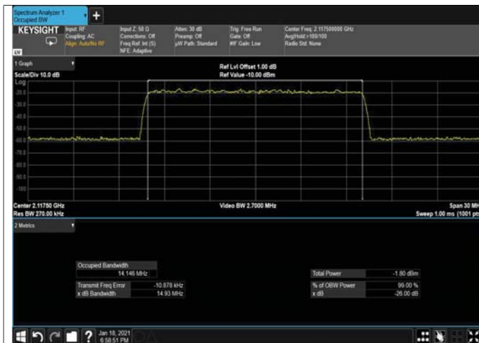
Figure 207: 64QAM 15MHz B.W; 2117.5MHz, 15kHz INPUT
