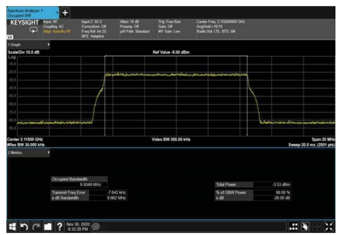
Figure 345: QPSK 10MHz B.W; 2115MHz – 4G INPUT
