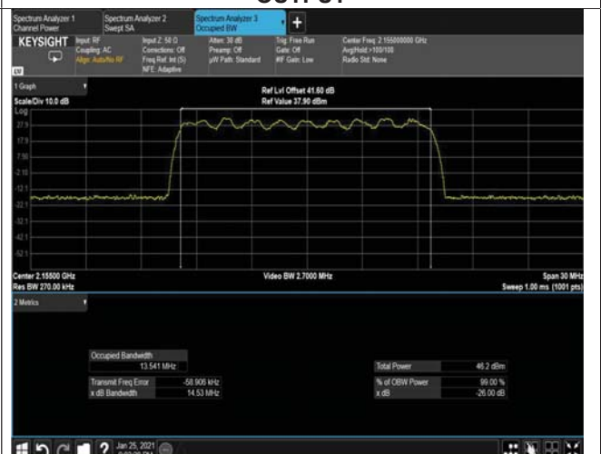
Figure 264: 16QAM 15MHz B.W; 2155.0MHz, 30kHz OUTPUT
