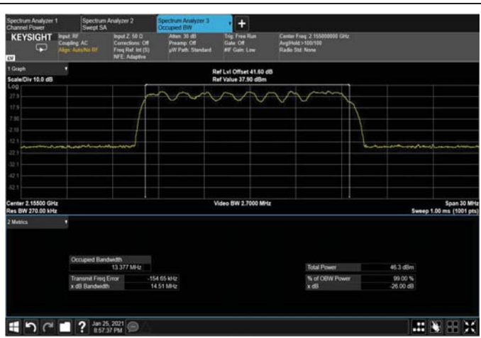
Figure 318: QPSK 15MHz B.W; 2155Hz, 30kHz OUTPUT
