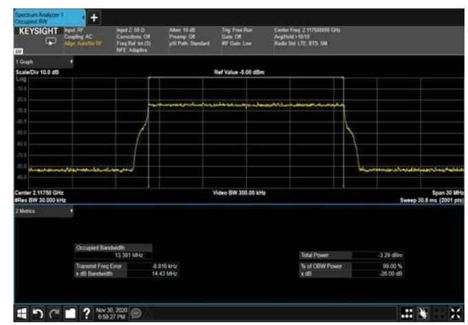
Figure 339: 64QAM 15MHz B.W; 2117.5MHz – 4G INPUT
