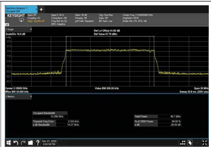
Figure 361: 16QAM 15MHz B.W; 2155MHz – 4G OUTPUT
