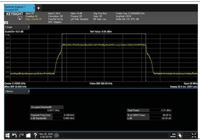
Figure 337: 64QAM 10MHz; 2155MHz – 4G INPUT
