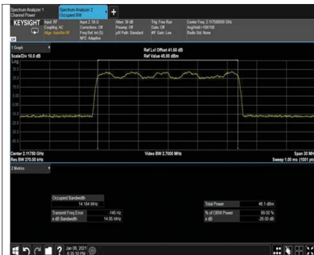
Figure 261: 16QAM 15MHz B.W; 2117.5MHz, 15kHz OUTPUT
