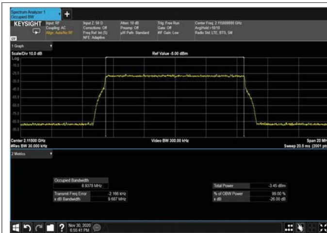
Figure 336: 64QAM 10MHz B.W; 2115MHz – 4G INPUT
