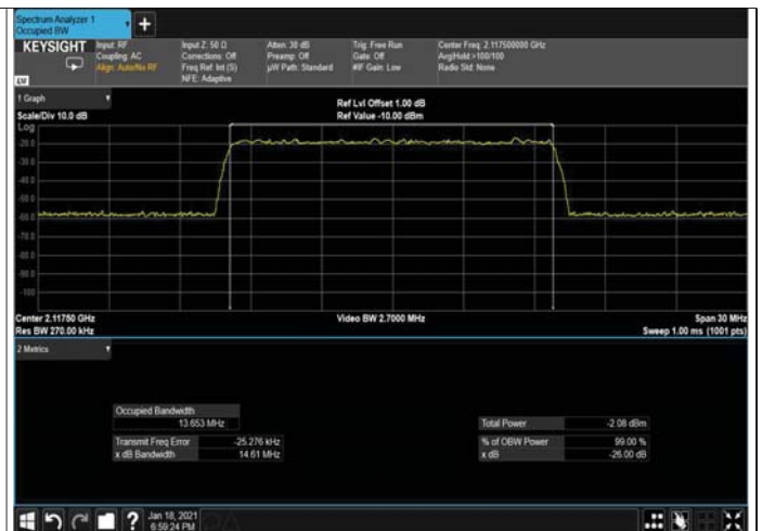
Figure 208: 64QAM 15MHz B.W; 2117.0MHz, 30kHz INPUT
