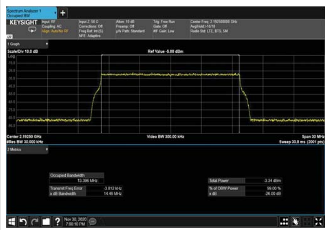
Figure 341: 64QAM 64MHz B.W; 2192.5MHz – 4G INPUT
