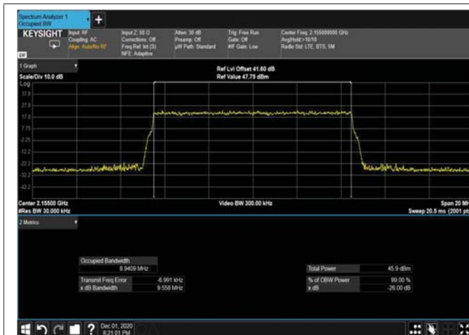
Figure 358: 16QAM 10MHz; 2155MHz – 4G OUTPUT
