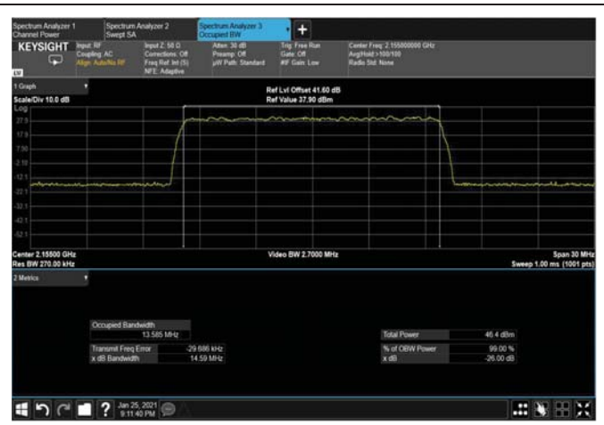
Figure 300: 256QAM 15MHz B.W; 2155MHz, 30kHz OUTPUT
