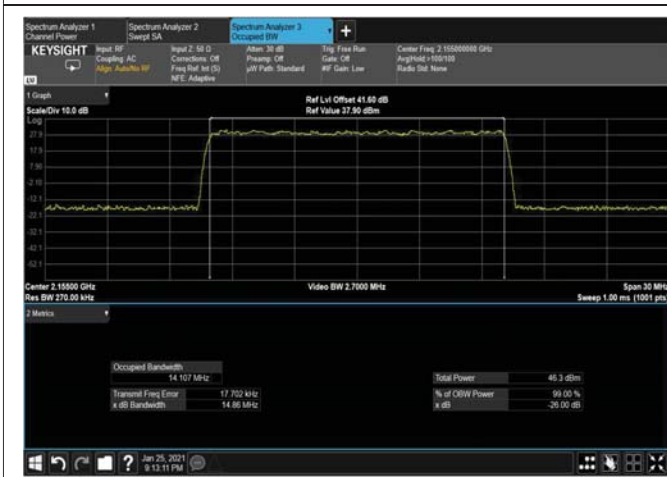
Figure 299: 256QAM 15MHz B.W; 2155MHz, 15kHz OUTPUT
