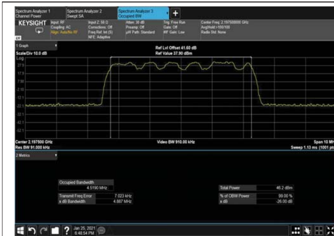
Figure 307: QPSK 5MHz B.W; 2197.5MHz, 15kHz OUTPUT
