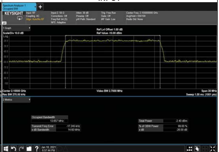
Figure 210: 64QAM 15MHz B.W; 2155.0MHz, 30kHz INPUT
