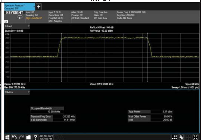
Figure 212: 64QAM 15MHz B.W; 2192.5MHz, 30kHz INPUT
