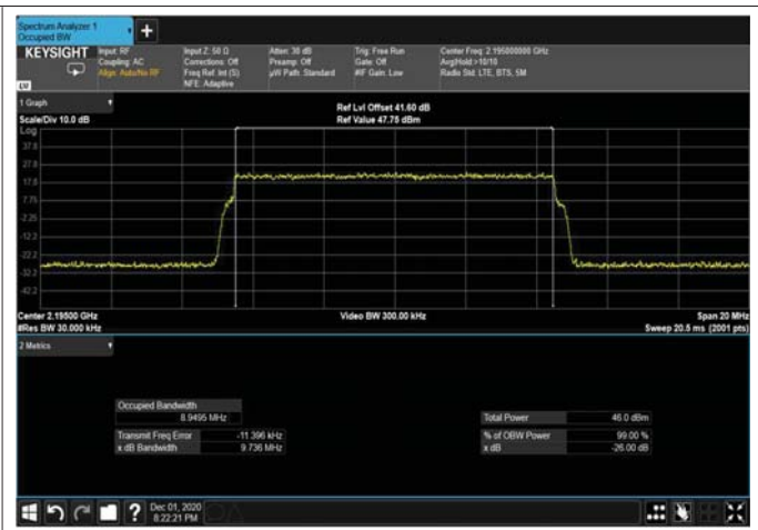
Figure 359: 16QAM 10MHz ; 2195MHz – 4G OUTPUT
