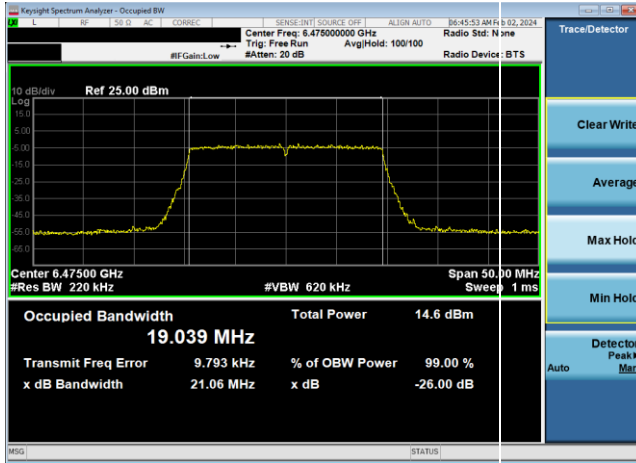
Plot 7-107. 26dB & 99% Bandwidth Plot Antenna WF8 (20MHz) 802.11ax (UNII Band 6) – Ch. 105, MCS11)
