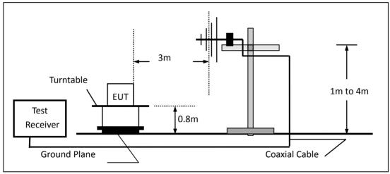
(c) For radiated emissions above 1000MHz
