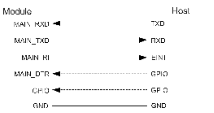
Figure 3: Sleep Mode Application via UART
