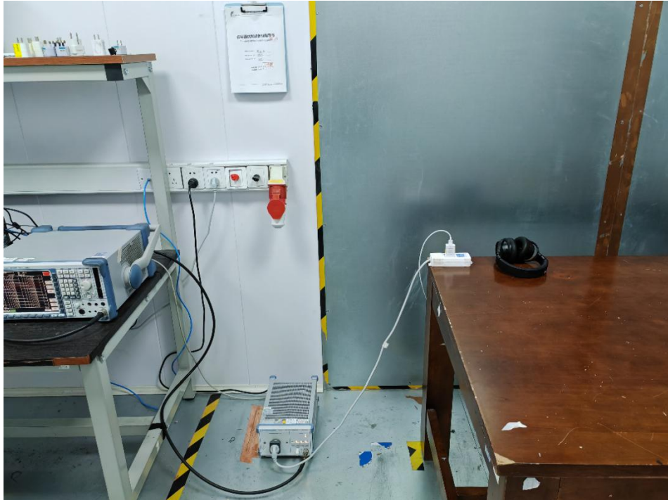
Conducted emissions at AC power line (150kHz-30MHz)
