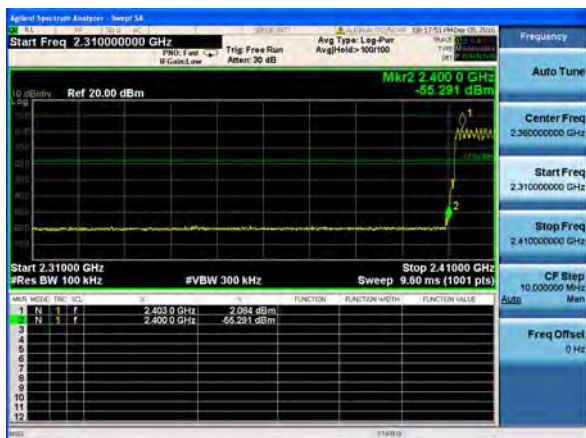
BDR mode (8DPSK): Band Edge-Low Channel (Hopping Mode)
