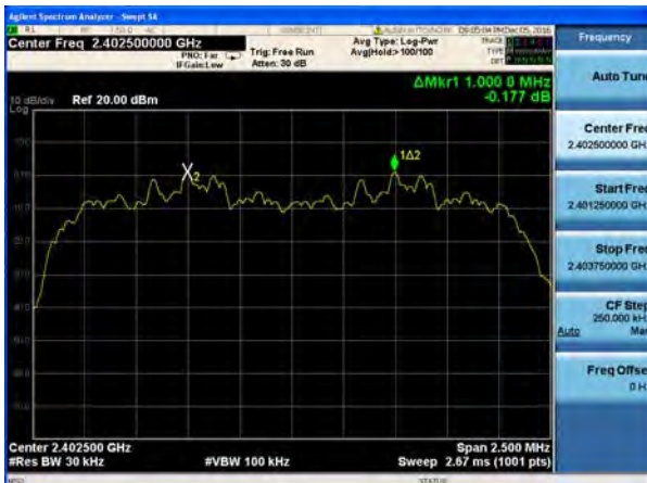
(2Mbps) Channel Separation plot on channel 39-40
