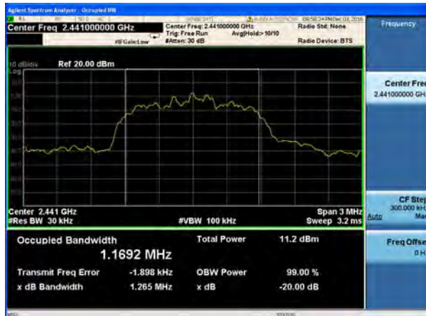
20dB Bandwidth plot on channel 78 (2Mbps)
