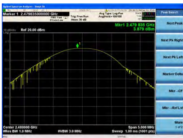
Peak output Power plot on channel 78 (1Mbps)
