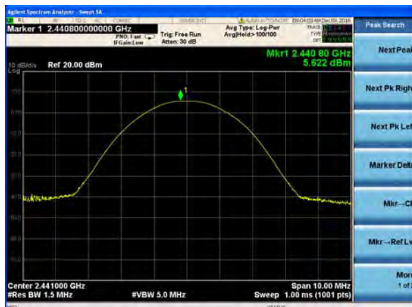
Peak output Power plot on channel 78 (2Mbps)
