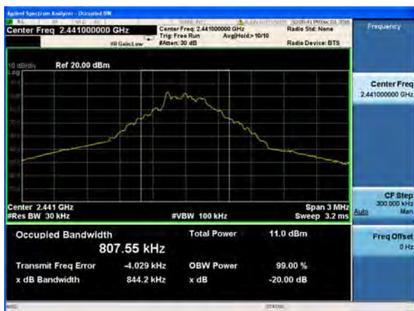
20dB Bandwidth plot on channel 78 (1Mbps)
