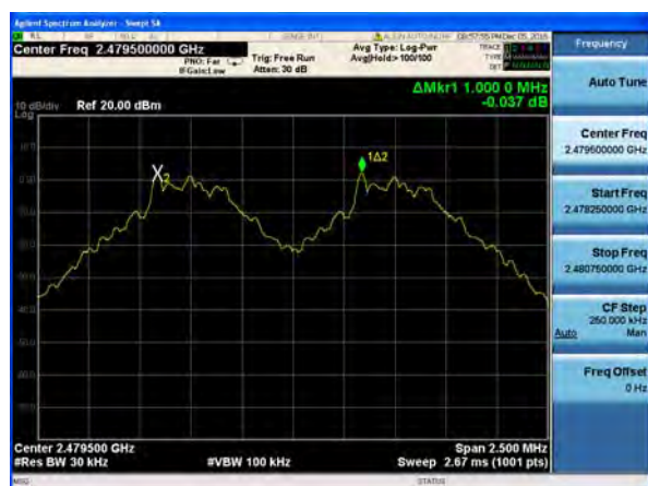
(1Mbps) Channel Separation plot on channel 77-78
