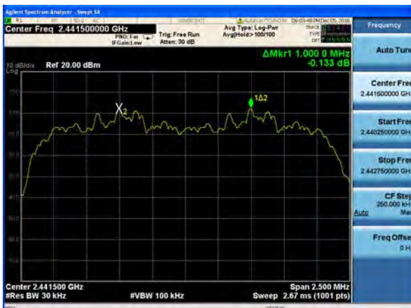
(2Mbps) Channel Separation plot on channel 77-78
