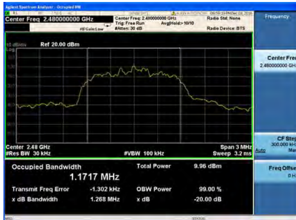
20dB Bandwidth plot on channel 78 (2Mbps)
