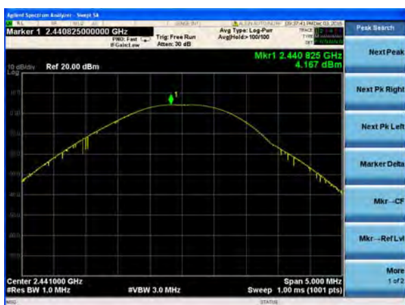
Peak output Power plot on channel 78 (1Mbps)
