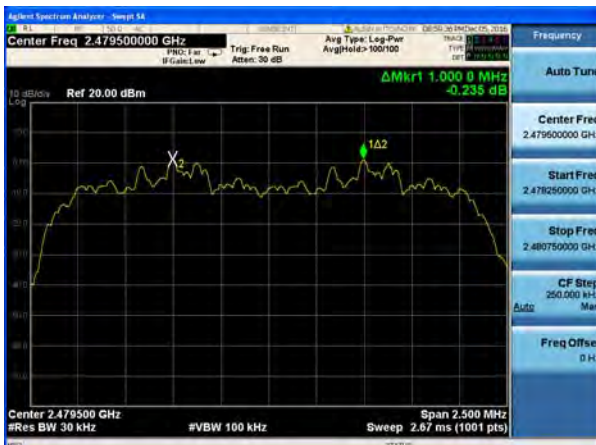
(2Mbps) Channel Separation plot on channel 77-78
