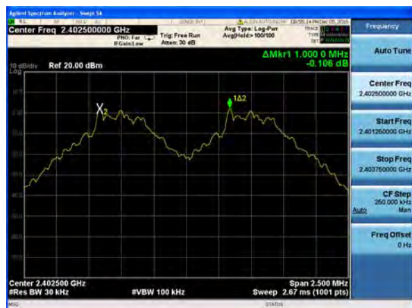
(1Mbps) Channel Separation plot on channel 39-40
