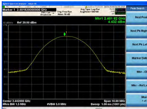
Peak output Power plot on channel 39 (2Mbps)
