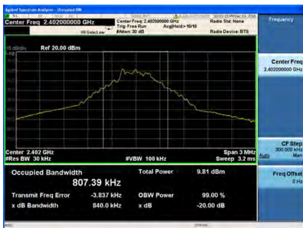
20dB Bandwidth plot on channel 39 (1Mbps)
