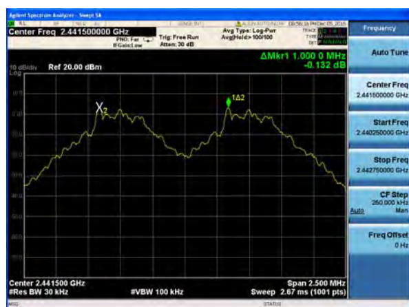
(1Mbps) Channel Separation plot on channel 77-78
