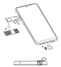
Caution: Do not insert the SIM pin into the speaker on top or bottom of the phone.
