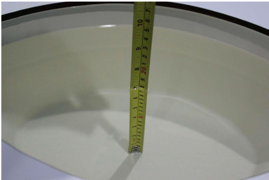
Picture 7-2: Liquid depth in the Flat Phantom(5GHz)
