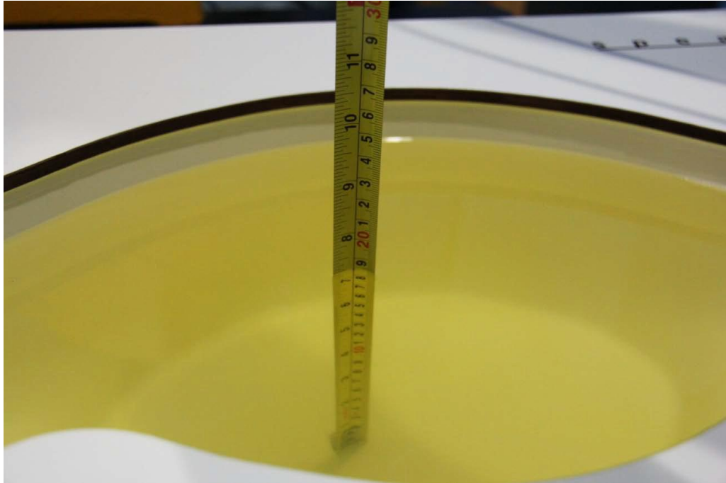
Picture 7-1: Liquid depth in the Flat Phantom(2450MHz)
