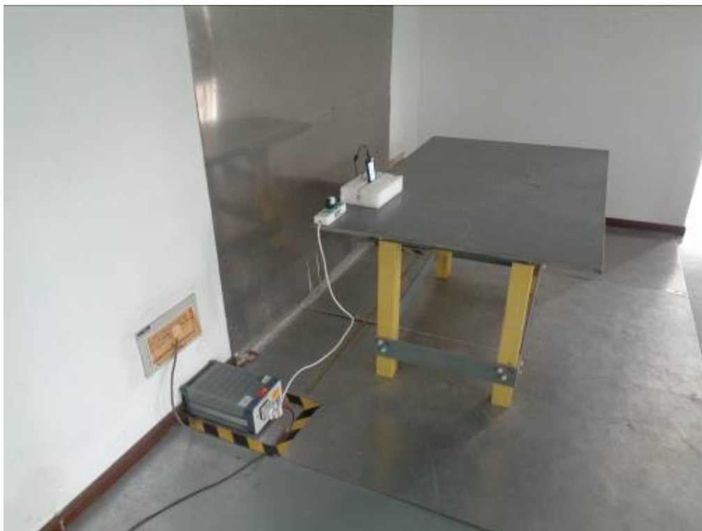
Conducted Emissions Test Setup – Side View
