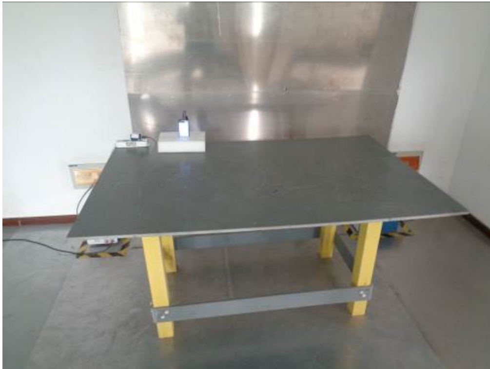
Conducted Emissions Test Setup – Front View
