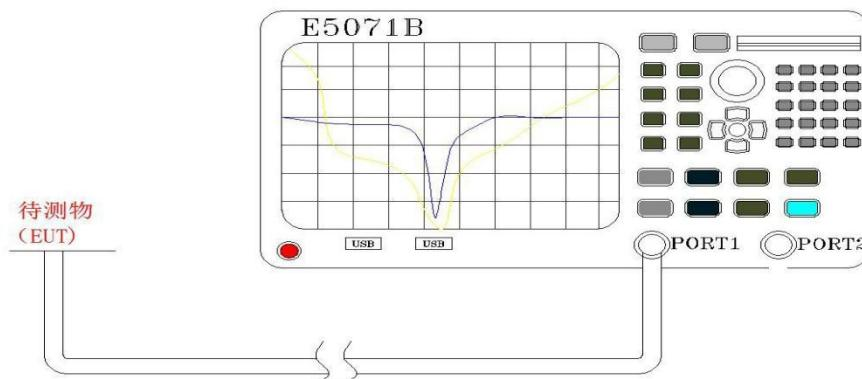
Fig.1 Antenna measured in Network Analyzer 图 1 天线测量网络分析仪
