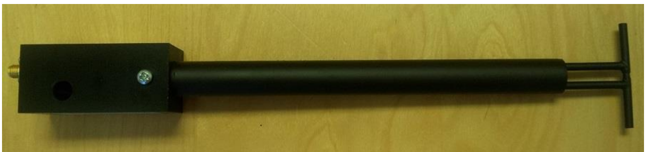
Figure 1 – MVG COMOSAR Validation Dipole
