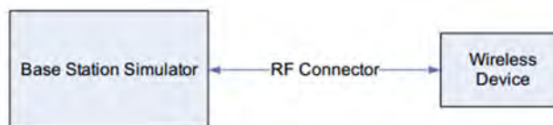
Figure 9.1 Power Measurement Setup
