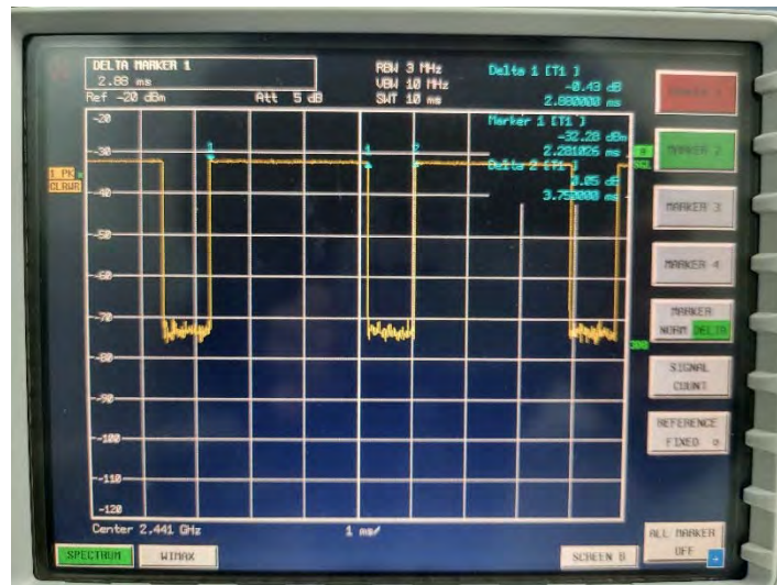
Figure 9.5.2 Bluetooth Transmission Plot
