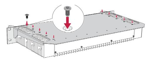
The chassis can be detached from the box and the inside parts become visible.
