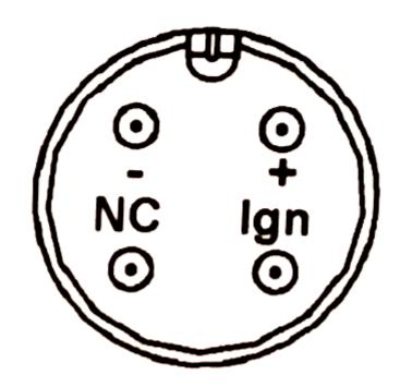
REMARK: When you don't have any intention to use the ignition signal, you need to connect the "Ign" pin to the +24v line in order for the unit to operate.
