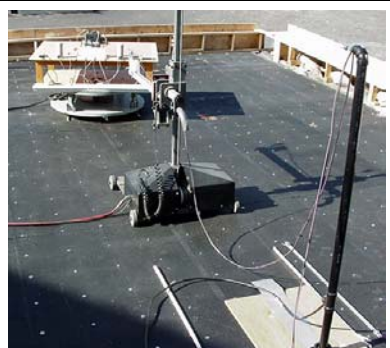
Photograph H-5 - Waveline Horn with LNA @ 1m
