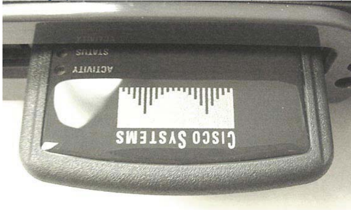
Photograph A-3 - WLAN Card Installed (cover removed)
