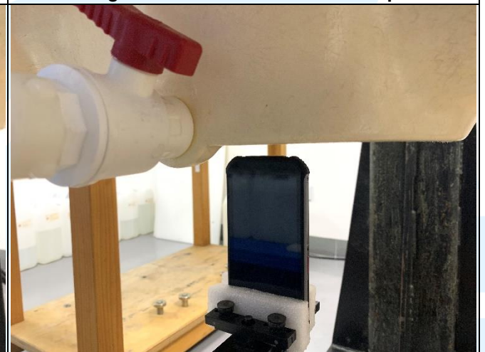
Bottom Side of EUT with 1.0 cm Gap
