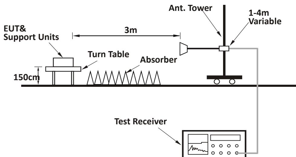
**TEST REPORT****7.4 Test Results of Radiated Emissions**
