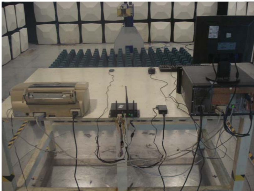
Radiated Emissions Test Setup - Rear View
