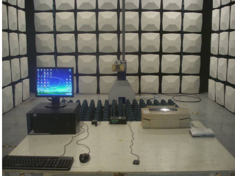
Radiated Emissions Test Setup - Front View
