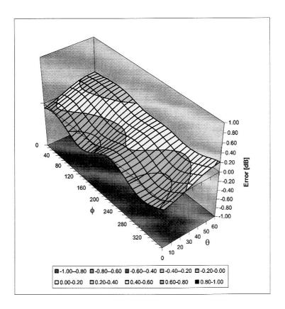
Spherical Isotropy Error < ± 0.4 dB
