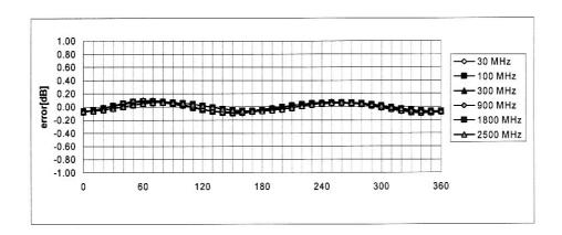
Axial Isotropy Error < ± 0.2 dB
