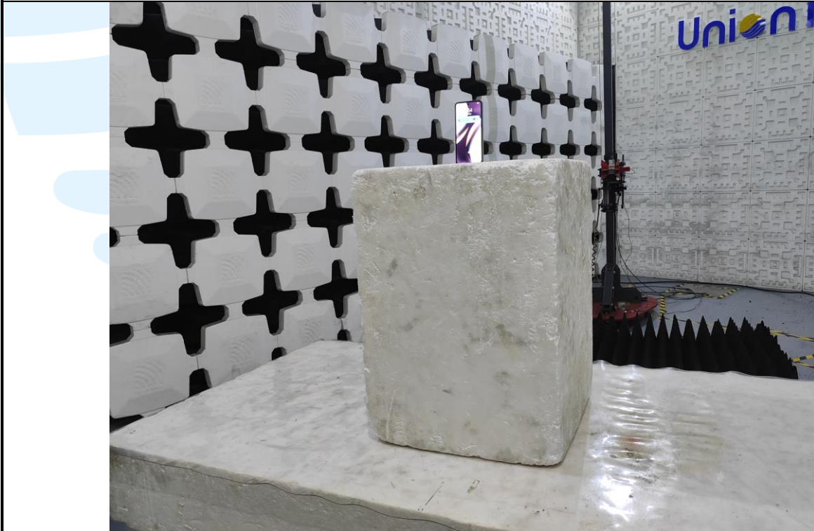
Radiated emission Test Setup (Above 1 GHz)
