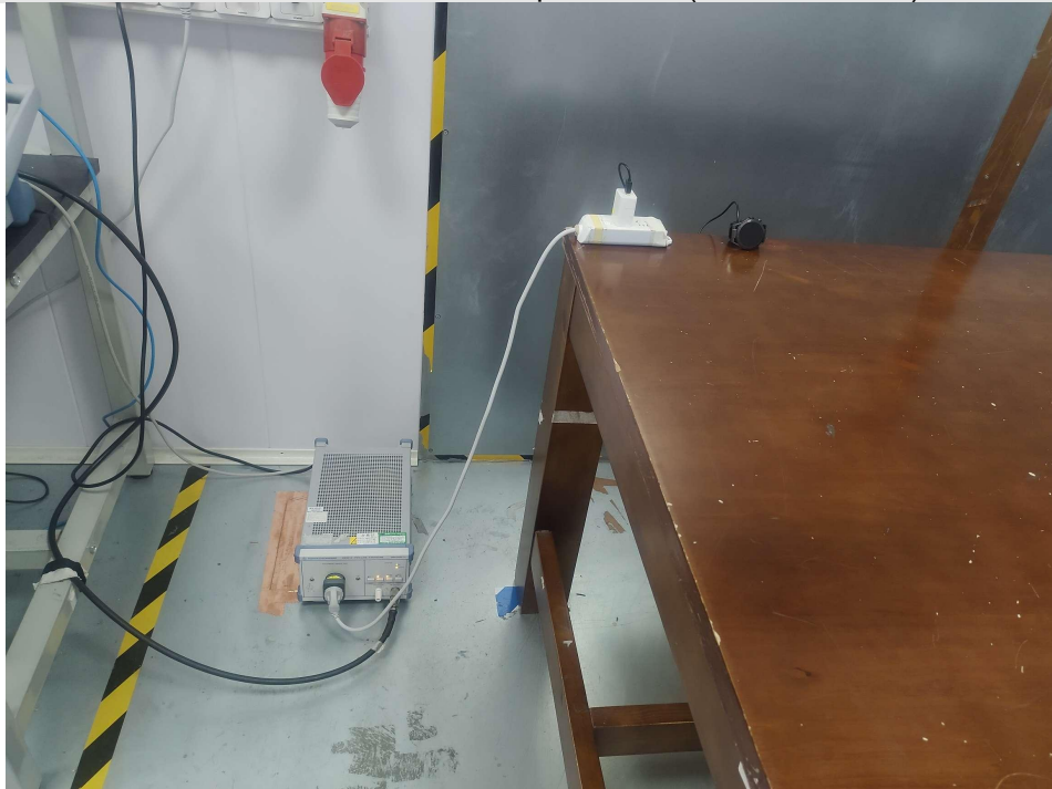
Conducted emissions at AC power line (150kHz-30MHz)
