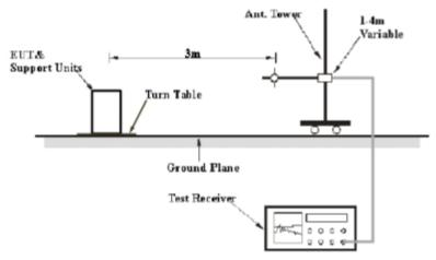
The radiated emission tests were performed in the 3-meter Chamber, using the setup accordance with the FCC part 2.1053. The specification used was the FCC 2.1053 limits. (dB):0dB
