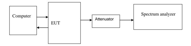
REMARKS: Attenuator loss (dB)=40dB, Cable Loss (dB)=1.5dB.
