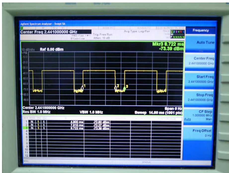
Time-domain plot for Bluetooth transmission signal
