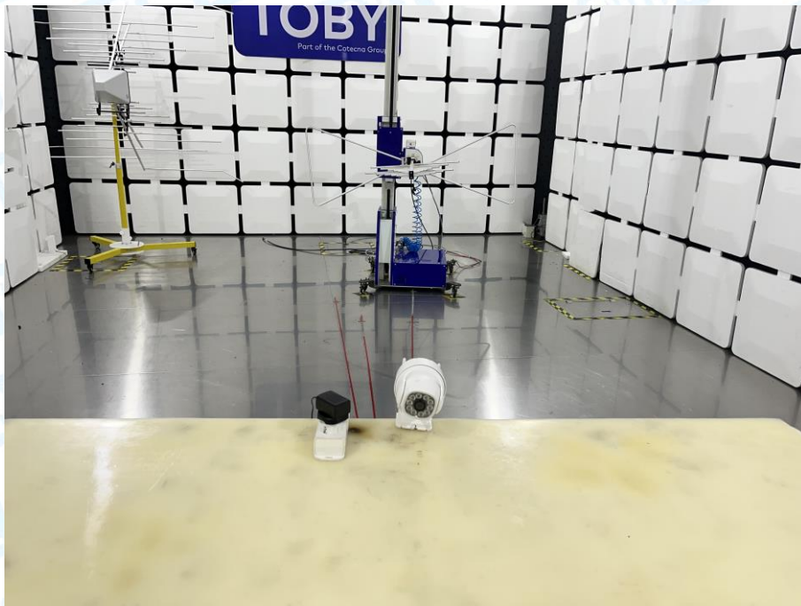
Photo of Setup for Radiated Emission (Below 1 GHz)-X20
